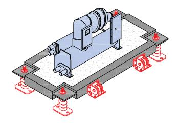
Inertia Pouring Frame has been developed for use with machines which produced high level of Vibration or those which are subjected to external forces or are simply unstable when mounted directly on high deflection/low stiffness helical spring or rubber Mountings for giving extremely high degree of vibration isolation without excessive motion.
